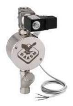
**P/N 0E39632 AISI 304 STAINLESS STEEL PULSER SINGLE VALVE (PSV) FOR ADBLUE® 1/2" WITH Y FILTER \*** AISI 304 stainless steel Pulser Single Valve version for AdBlue® with G 1/2" (f) connections. Max working pressure 16 bar.
