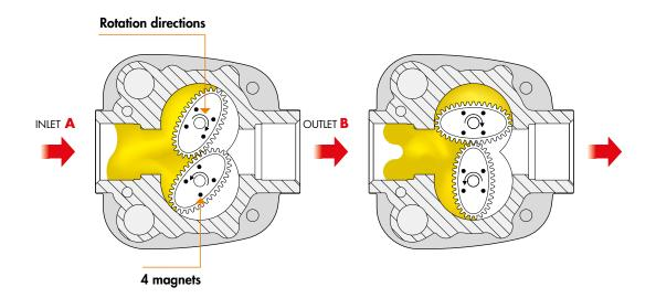
When the fluid enter in the oval gear chamber through the inlet "A", the gears start to rotate.
