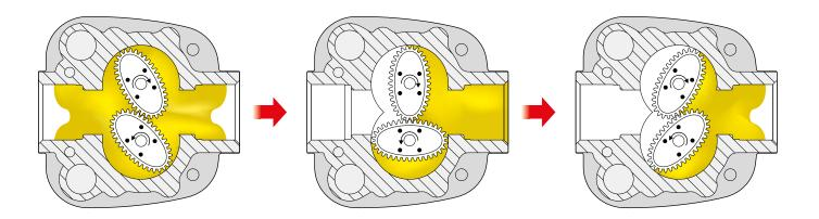
Correct dimensional tollerances between gears and chamber grant the reliability and the accuracy of the meter.
